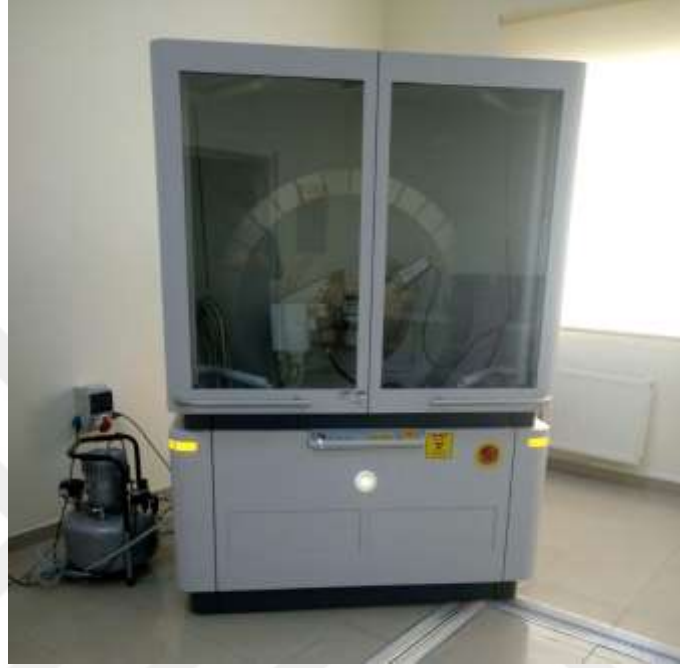
Şekil 3.4. Panalytical Marka empyrean model XRD
